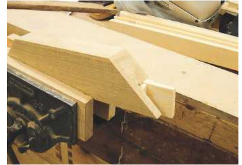
▲ Pic.15 A simple mitre block is used to guide the chisel...
